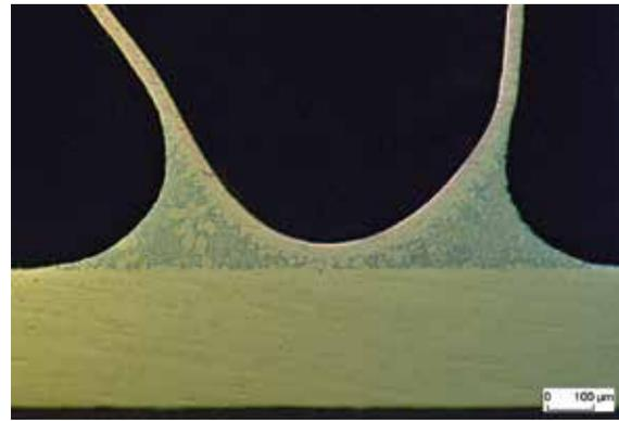
A micrograph of a tube-fin joint of a copper-based heat exchanger brazed with VITROBRAZE VZ2255
